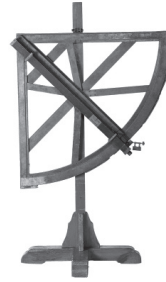
Figure 2: Inō Tadataka's quadrant used to measure latitude Courtesy of the Inō Tadataka Museum, Katori City, Chiba, Japan
